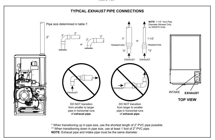
Figure 23. Typical Exhaust Pipe Connections
