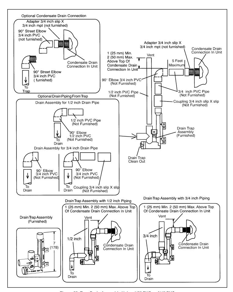
Figure 52. Trap Drain Assembly Using 1/2" PVC or 3/4" PVC
