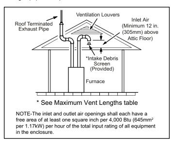
Figure 7. Equipment in Confined Space (Inlet Air from Ventilated Attic and Outlet Air to Outside)
