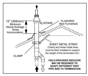
Figure 35. Direct Vent Concentric Rooftop
