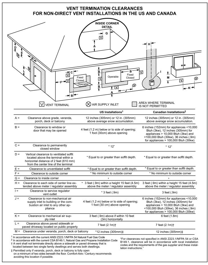
Figure 29. Vent Termination Clearances for Non-Direct Vent Installations
