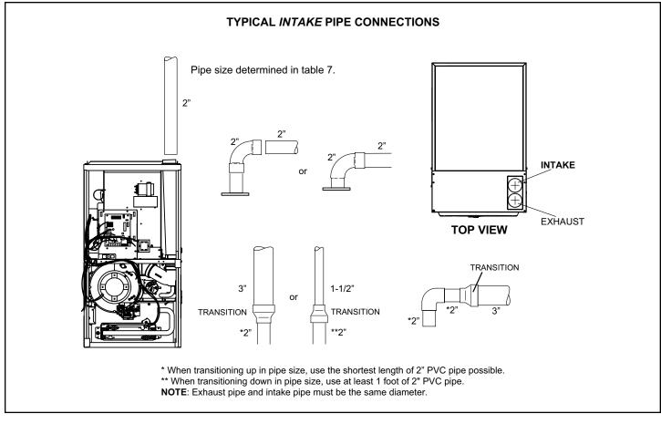
Figure 24. Typical Intake Pipe Connections (Direct Vent Applications)
