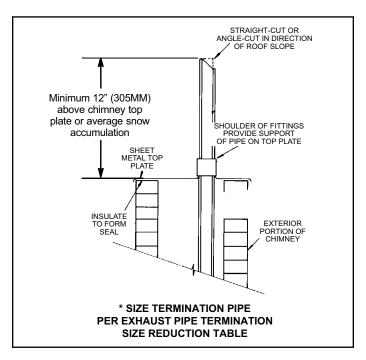
Figure 43. Non-Direct Vent Application Using Existing Chimney
