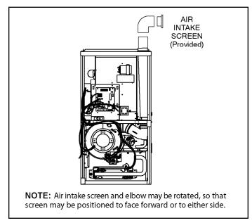
Figure 25. Typical Air Intake Pipe Connections
