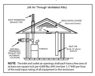
Figure 9. Equipment in Confined Space - All Air from Outside
