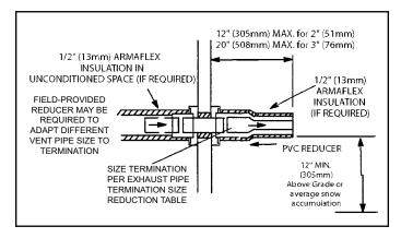
Figure 41. Non-Direct Vent Field Supplied Wall Termination
