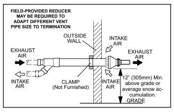
Figure 36. Direct Vent Concentric Wall Termination
