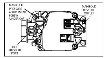
Figure 61. Gas Valve Shown in "ON' Position
