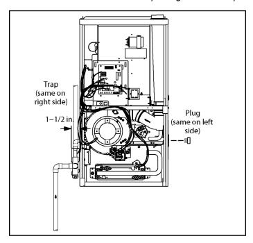
Figure 47. Condensate Trap and Plug Locations
