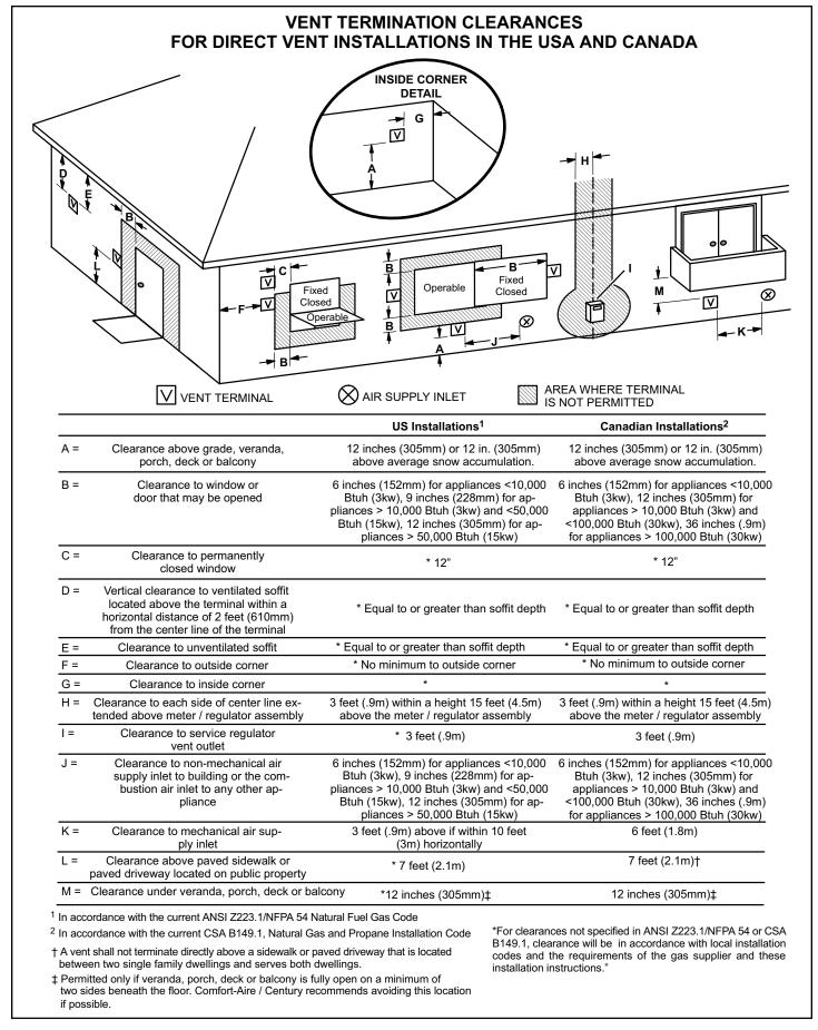
Figure 30. Vent Termination Clearances for Direct Vent Installations
