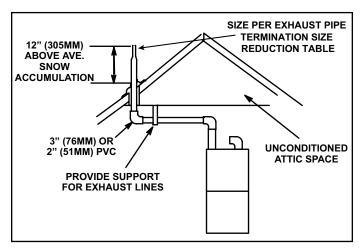
Figure 40. Non-Direct Vent Roof Termination Kit
