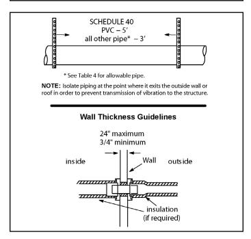
Figure 20. Piping Suspension Guidelines
