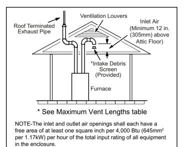
Figure 26. Equipment in Confined Space (Inlet Air from Ventilated Attic and Outlet Air to Outside)
