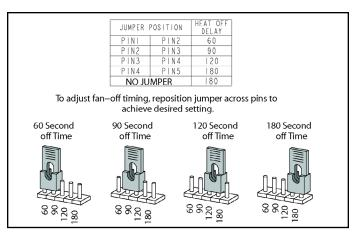
Figure 62. Heat Fan-OFF Time in Seconds
