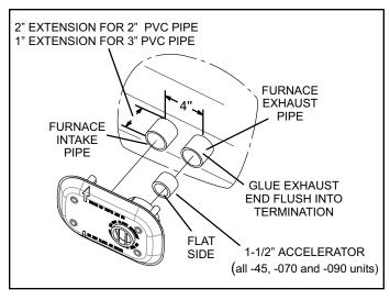
Figure 34. Flush Mount Side Wall Termination
