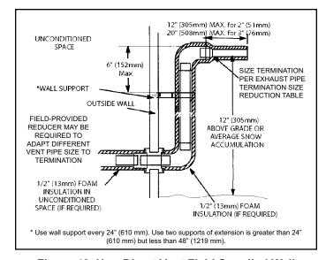
Figure 42. Non-Direct Vent Field Supplied Wall Termination Extended
