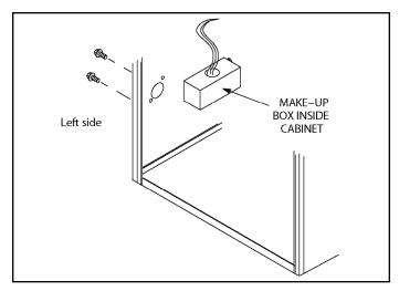
Figure 55. Interior Make-Up Box (Factory - Installed Left Side)
