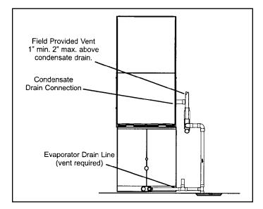
Figure 50. Evaporator Coil Using a Common Drain
