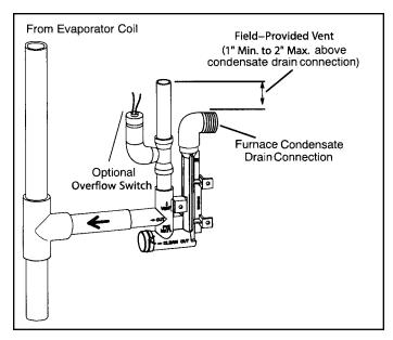
Figure 51. Condensate Trap with Optional Overflow Switch
